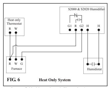
Connect field wiring as shown in Figures 5 or 6.
